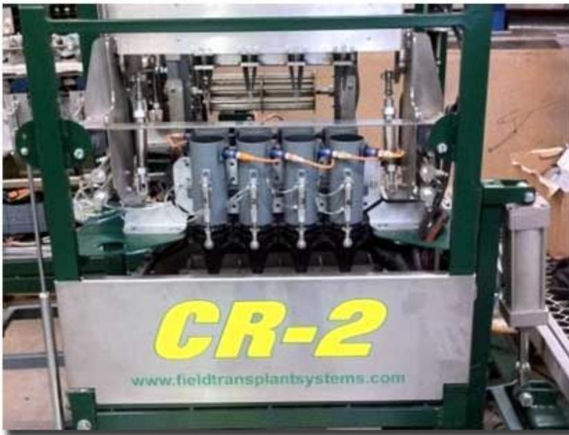
This machine is what we refer to as a selector model. (CR2) It will ensure planted rows are complete with a full complement of plants .. no misses. It does this by optical sensor recognising when the picking fingers prove a seed has not germinated in the cellular tray. The plant receiving cup will remain closed while another opens to deliver a held seedling to the planting shoe. The function is repetitive and continuous. Our automatic planters are offered with or without the selector. device.
