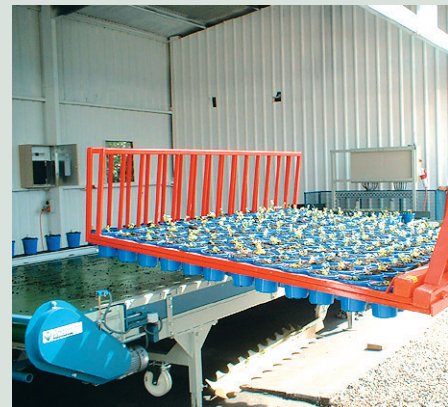
At Payneham Plant Wholesalers in South Australia, pots are moved in bulk following the installation of a Buffer Table System.
